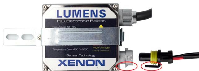
8. Connect the other end of the connector from ballast to vehicle's factory headlight socket (the one you unplugged from the original headlight bulb). Some connectors are pre-pinned, but be sure to check and ensure that the black wire is connected to the ground wire on the factory harness and the red / blue wire is connected to the positive wire on the factory harness. If these wires are reversed, the HID's will not power on - simply reverse the pins.
